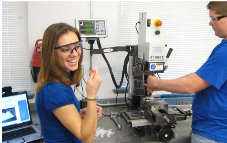
Figure 3. Students using a milling / drilling machine to fabricate a centrifugal pump.
