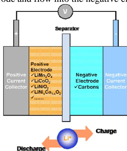
Figure 1 Schematic of the lithium ion battery operation
