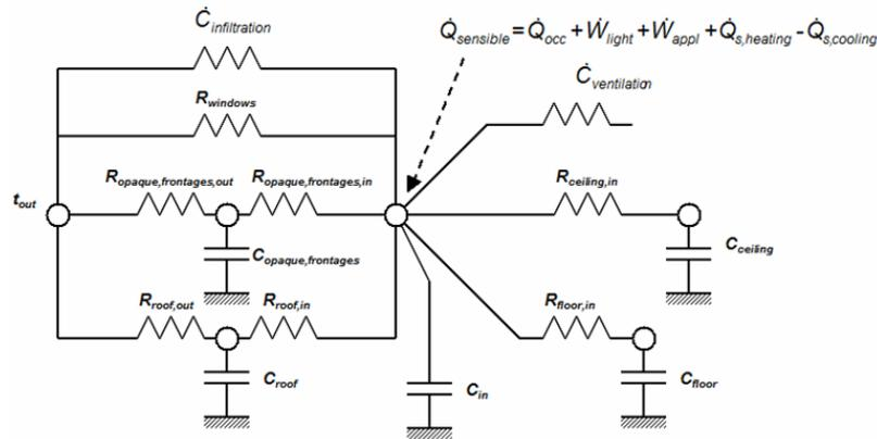
Figure 2: Simplified building simulation model
