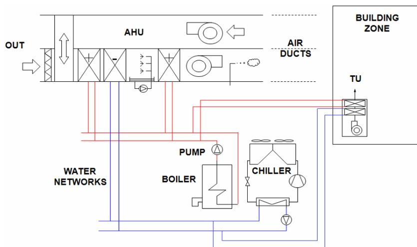
Figure 3: The HVAC system considered in BENCHMARK
